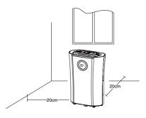
excessive moisture as soon as it is turned on. Excess moisture is dispersed throughout your home. For this reason, the dehumidifier should be positioned in a central and clear location so that it can draw this moist air towards it from all over the home. A warm hallway or landing is an excellent position for your dehumidifier. If possible, leave interior doors ajar to allow air circulation.
