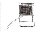
Make sure the connection between pipe and the drain outlet is tight and does not leak. Then direct the pipe to a suitable drainage point. This unit uses gravity to dispose of water hence the drain should be lower than the water outlet on the unit. Put the tank back. Be sure to run the water pipe downward and let the water to flow out smoothly. Do not kink or bend the pipe.
